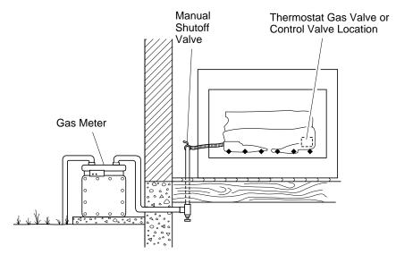
Figure 15 - Checking Gas Joints
